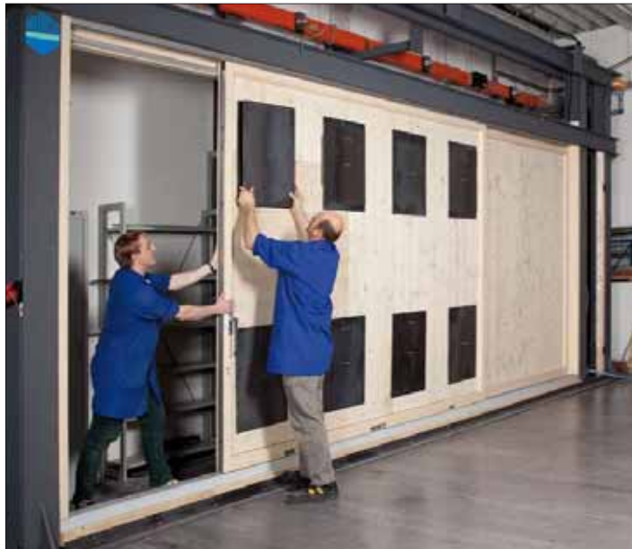
MACO fatigue test carried out on a 400 kg Lift & Slide unit with a sash thickness of 30085 mm and a frame width of 6800 mm at MACO's internal test centre in Salzburg; the sash weight is reproduced through applied metal plates. The operating intervals correspond to the standards set by accredited testing institutes.
